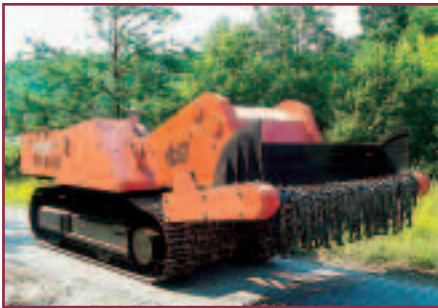
RM-KA 02 remote-controlled flail. ©Duro Dakovic Specialjalna Vozila
